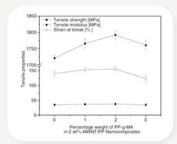
PP was diluted by PP SP179 (copolymer, Izod notched impact strength is about (40~45 KJ/m2) using a twinscrew extruder, then the specimens were made by Injection molding.
